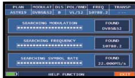
DIE "HELP" FUNKTION VERSUCHT DIE EMPFANGSPARAMETER DES DIGITALEN SIGNALS ZU ERMITTELN.
