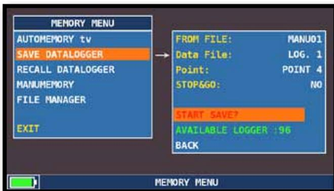
NAVIGIEREN SIE AUF "SAVE DATALOGGER" SETZEN SIE DIE GEWÜNSCHTEN PARAMETER UND WÄHLEN SIE "START SAVE?" UM EINE NEUE LOGGER-DATEI ZU GENERIEREN.
